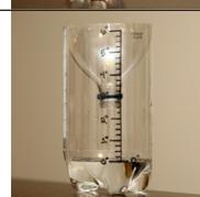
Be sure to place your rain gauge in an open area, away from water that could drop from a roof or from trees.
